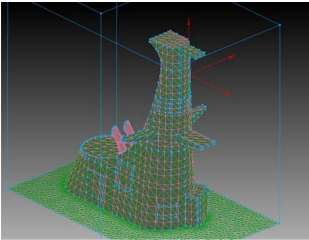
**Figure 3:** CFD surface mesh created using Pointwise.
